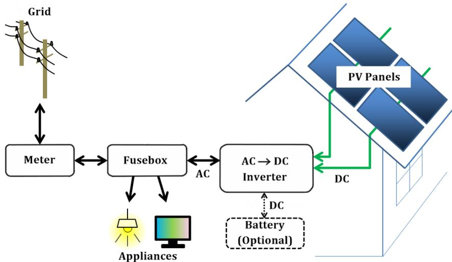
**Figure 2.2:** Typical grid-tied PV system.
