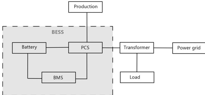
**Figure 2.25:** Simplified overview of a BESS and surrounding system components.
