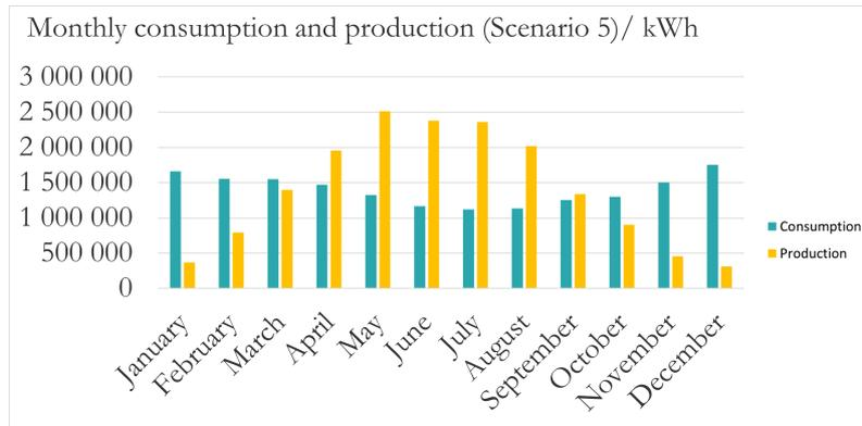
**Figure 4.27:** Monthly production and consumption for Scenario 5: Shore power with 16.3 MW PV.
