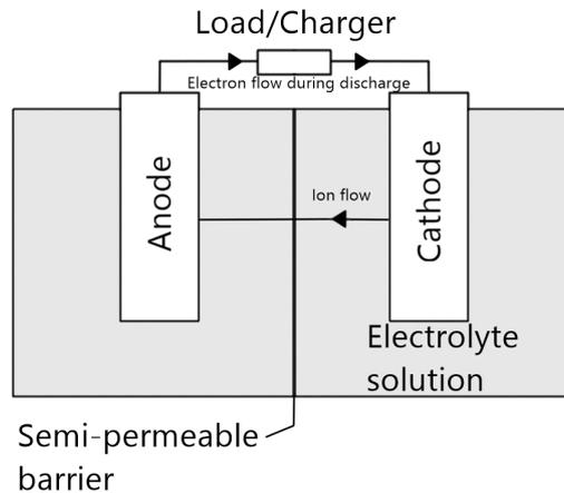
**Figure 2.23:** Schematic drawing of a battery.
