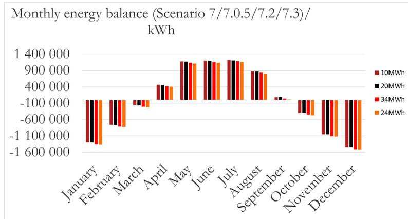
**Figure 4.38:** Monthly energy balance for Scenario 7/7.0.5/7.1/7.2: Shore power with 16.3 MW PV with 10 MWh, 20 MWh, 34 MWh and 24 MWh battery.
