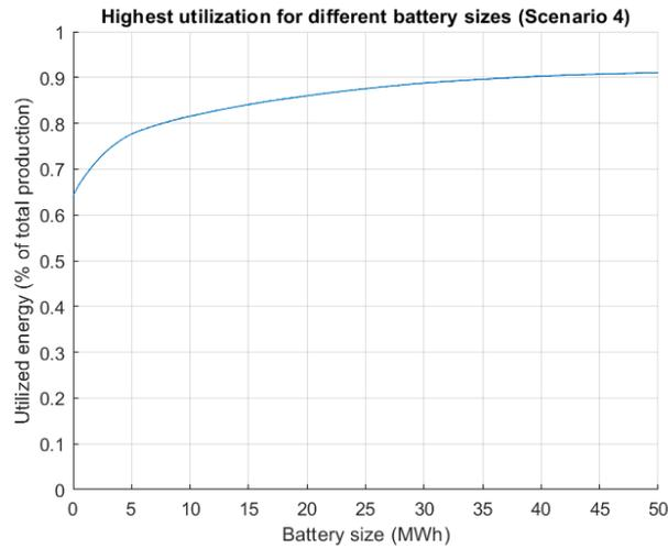
Figure 4.19: Highest utilization for each battery size.
