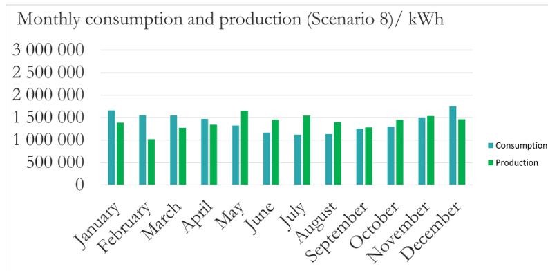
**Figure 4.44:** Monthly production and consumption for Scenario 8/8.0.5/8.1/8.2: Shore power with 4.6 MW PV and 3 MW Wind with a battery.
