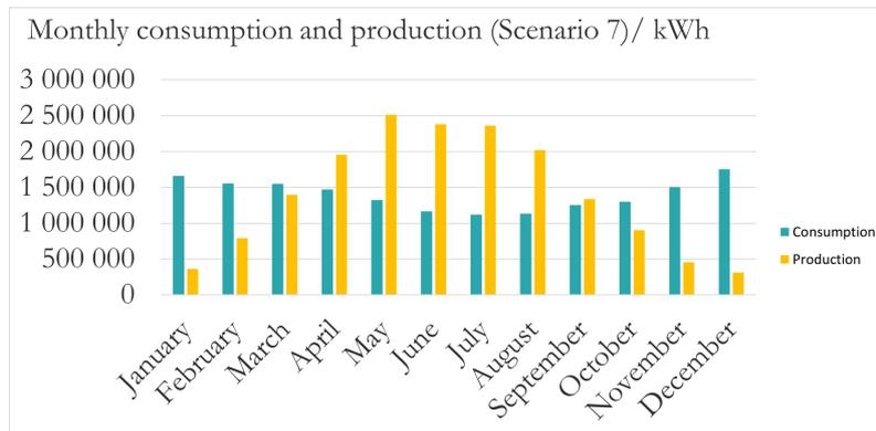
**Figure 4.37:** Monthly production and consumption for Scenario 7/7.0.5/7.1/7.2: Shore power with 16.3 MW PV with a battery.
