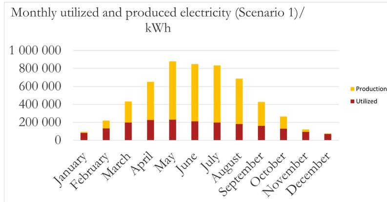
**Figure 4.8:** Monthly production with the amount of utilized electricity of the production for Scenario 1: Current consumption with 5.7 MW PV.
