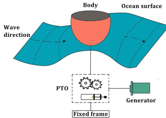
**Figure 2.18:** Basic principle of OBWAEC technology.
