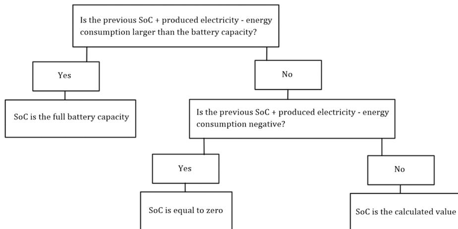
**Figure 3.10:** Sketch of the logic used for state of charge in Excel.
