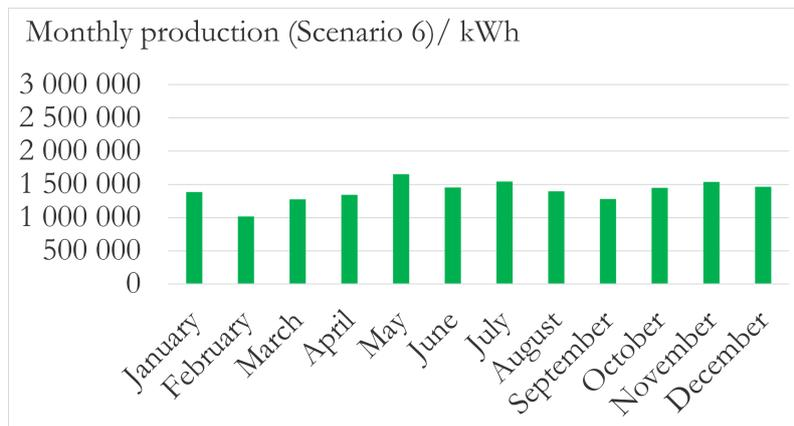
**Figure 4.31:** Monthly production for Scenario 6: Shore power with 4.6 MW PV and 3 MW Wind.
