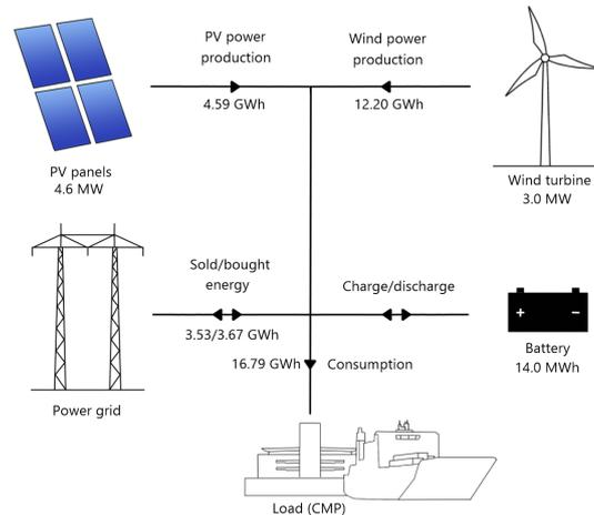
**Figure 6.2:** Overview of the system with the highest utilization for the shore power scenario (Scenario 8.0.5). Energy flows and capacity are presented with arrows representing energy flow directions.
