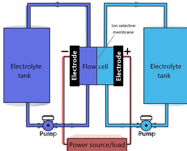
Figure 2.24: Schematic image of a flow battery.
