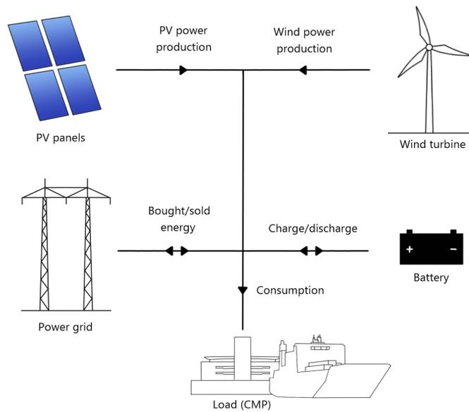
**Figure 3.9:** Overview of the energy flows in the complete system. Arrows represent energy flow directions.
