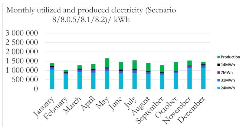
**Figure 4.46:** Monthly production with the amount of utilized electricity of the production for Scenario 8/8.0.5/8.1/8.2: Shore power with 4.6 MW PV and 3 MW Wind with 7 MWh, 14 MWh, 31 MWh and 24 MWh battery.
