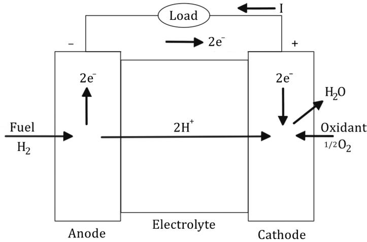
**Figure 2.27:** The simple operation of a fuel cell.
