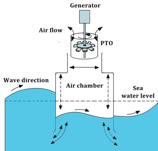
**Figure 2.19:** Basic principle of OWCWAEC technology.
