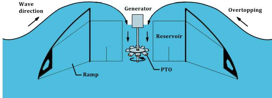
**Figure 2.20:** Basic principle of OWAEC technology.
