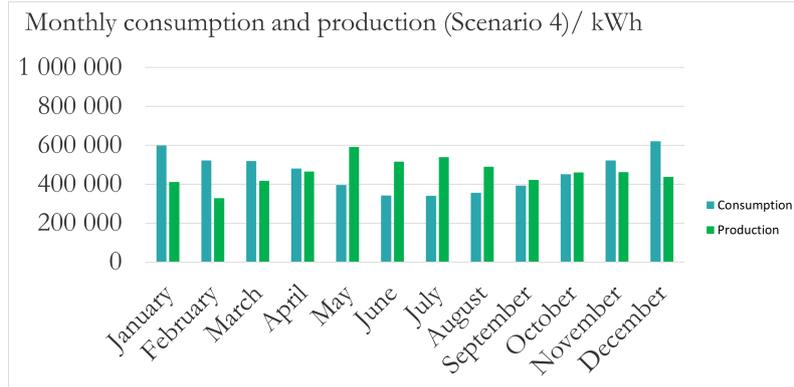
**Figure 4.22:** Monthly production and consumption for Scenario 4/4.0.5/4.1/4.2: Current consumption with 2.1 MW PV and 1.0MW Wind with a battery.
