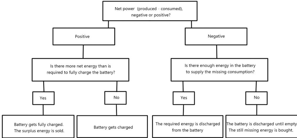
**Figure 3.8:** Sketch of the logic used when determining charge and discharge from the battery as well as when to buy and sell energy.
