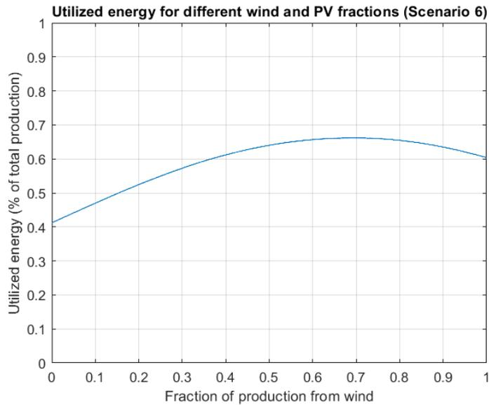
**Figure 4.30:** Utilized energy as a function of the fraction of electricity produced by wind. 100% wind energy corresponds to wind power producing energy equaling the yearly consumption. Solar power produces the fraction that wind doesn't produce.
