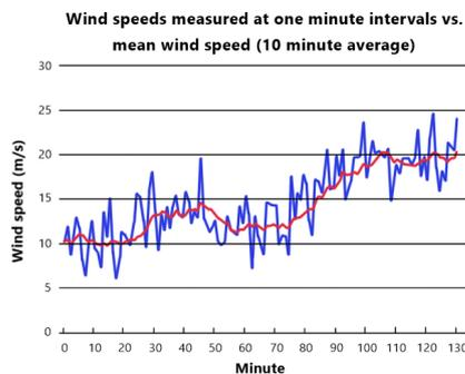
**Figure 2.16:** Measured wind speeds (Blue) plotted together with 10 minute mean wind speeds (Red).
