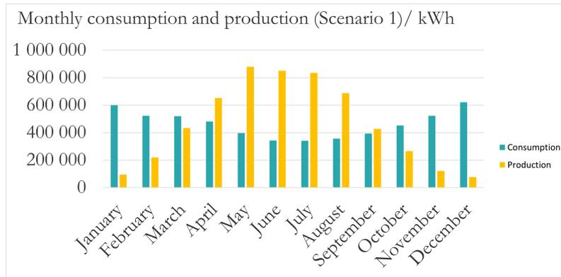
**Figure 4.6:** Monthly production and consumption for Scenario 1: Current consumption with 5.7 MW PV.
