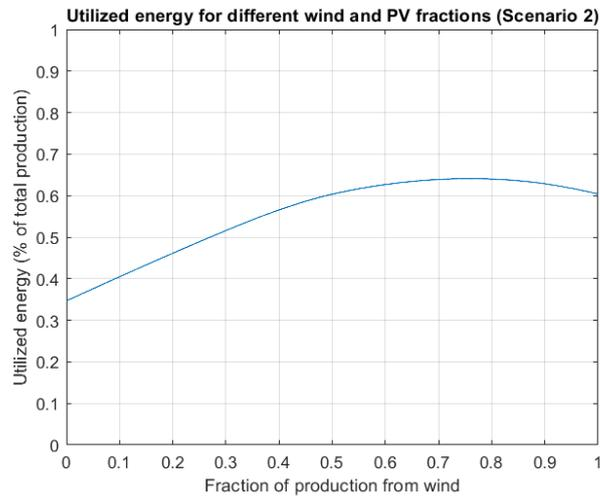
**Figure 4.9:** Utilized energy as a function of the fraction of electricity produced by wind. 100% wind energy corresponds to wind power producing energy equaling the yearly consumption. Solar power produces the fraction that wind doesn't produce.
