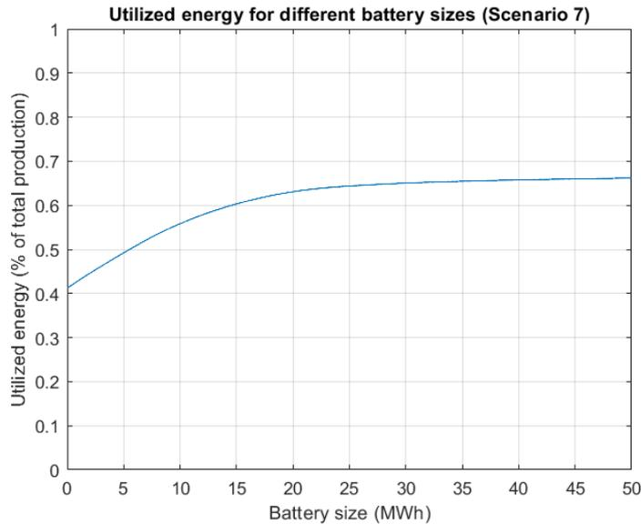
**Figure 4.35:** Utilized energy as a function of battery size.
