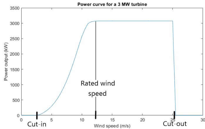
**Figure 2.10:** Example of a power curve with marked cut-in and cut-out wind speeds. Curve represents a 3 MW turbine.
