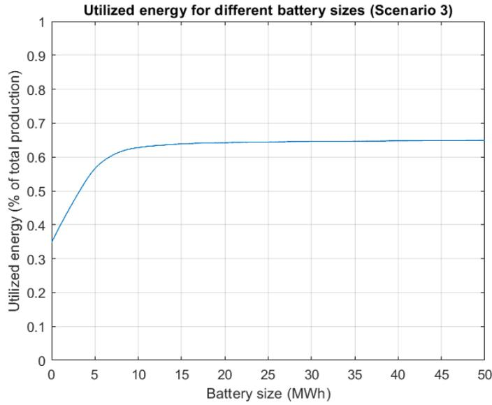
**Figure 4.14:** Utilized energy as a function of battery size.
