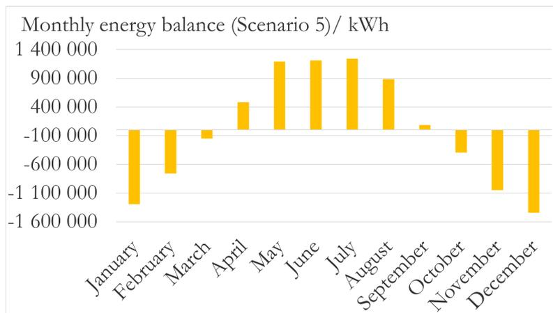
**Figure 4.28:** Monthly energy balance for Scenario 5: Shore power with 16.3 MW PV.
