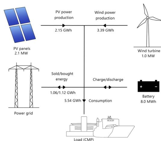
**Figure 6.1:** Overview of the system with the highest utilization for the current consumption scenario (Scenario 4.0.5). Energy flows and capacity are presented with arrows representing energy flow directions.
