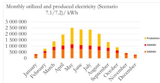
**Figure 4.40:** Monthly production with the amount of utilized electricity of the production for Scenario 7.1/7.2: Shore power with 16.3 MW PV with 34 MWh and 24 MWh battery.
