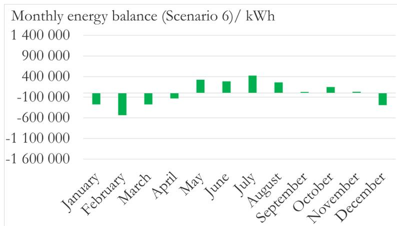
**Figure 4.33:** Monthly energy balance for Scenario 6: Shore power with 4.6 MW PV and 3 MW Wind.
