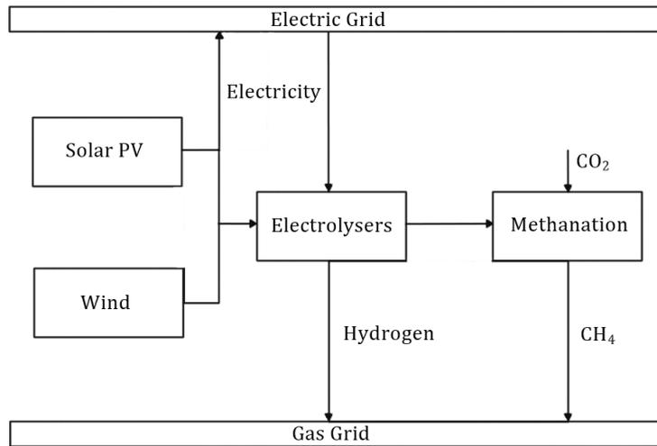
**Figure 2.28:** The principle of power-to-gas.
