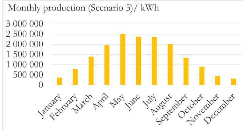
**Figure 4.26:** Monthly production for Scenario 5: Shore power with 16.3 MW PV.
