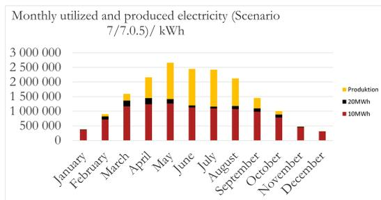
**Figure 4.39:** Monthly production with the amount of utilized electricity of the production for Scenario 7/7.0.5: Shore power with 16.3 MW PV with 10 MWh and 20 MWh battery.
