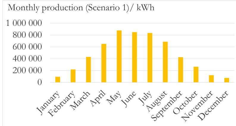
**Figure 4.5:** Monthly production for Scenario 1: Current consumption with 5.7 MW PV.
