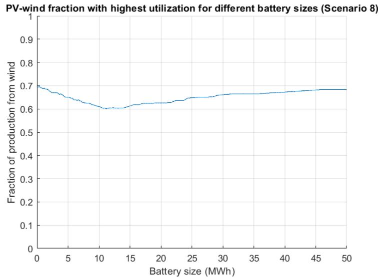
**Figure 4.42:** Fraction of production from wind resulting in the highest utilization as a function of battery size.
