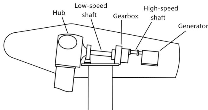
**Figure 2.11:** Schematic drawing of the components in a wind turbine with gearbox.
