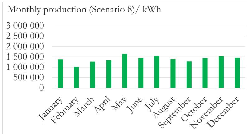
**Figure 4.43:** Monthly production for Scenario 8/8.0.5/8.1/8.2: Shore power with 4.6 MW PV and 3 MW Wind with a battery.
