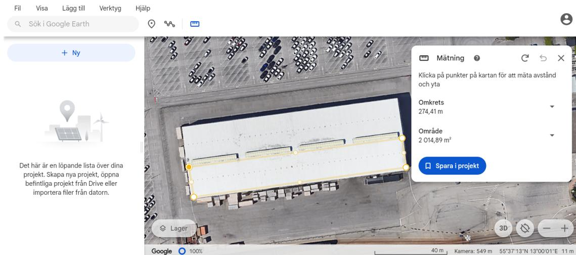
Figure 3.2: Example of measurement technique used in Google Earth.
