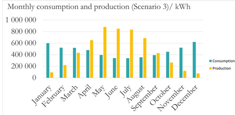
**Figure 4.16:** Monthly production and consumption for Scenario 3/3.0.5/3.1/3.2: Current consumption with 5.7 MW PV with a battery.
