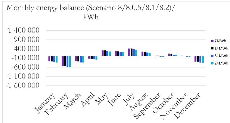
**Figure 4.45:** Monthly energy balance for Scenario 8/8.0.5/8.1/8.2: Shore power with 4.6 MW PV and 3 MW Wind with 7 MWh, 14 MWh, 31 MWh and 24 MWh battery.
