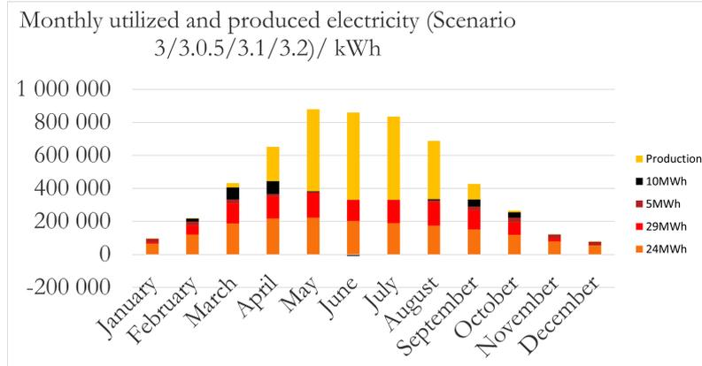
**Figure 4.18:** Monthly production with the amount of utilized electricity of the production for Scenario 3/3.0.5/3.1/3.2: Current consumption with 5.7 MW PV with 5 MWh, 10 MWh, 29 MWh and 24 MWh battery.
