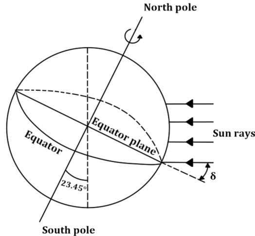
**Figure 3.4:** Definition of declination angle
