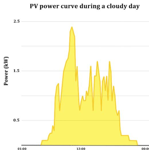
**Figure 2.9:** Power curve from a 4.2kW PV system during a cloudy day. Data taken from [15]
