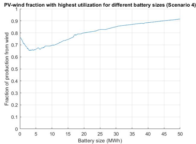
Figure 4.20: Fraction of production from wind resulting in the highest utilization as a function of battery size.
