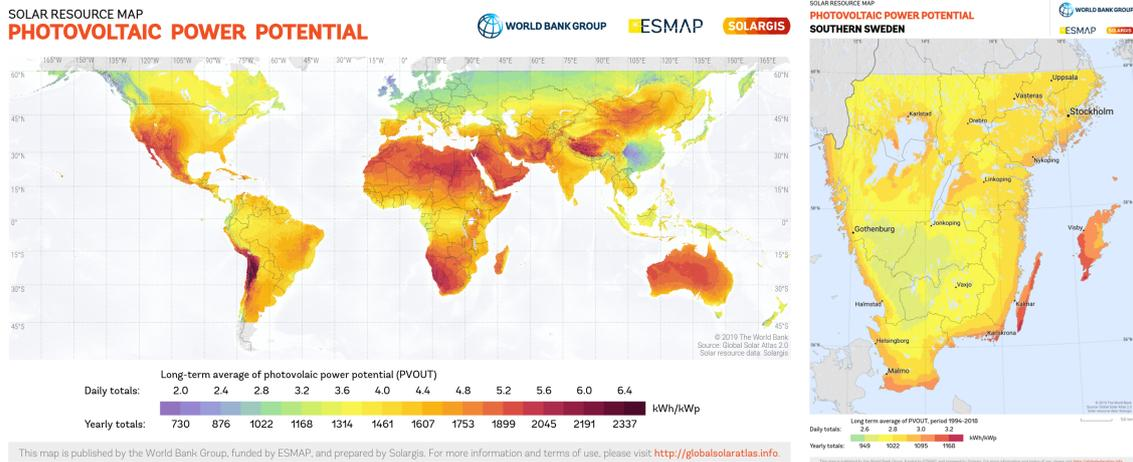
**Figure 2.5:** PV power potential in the world and specifically southern Sweden. The text in the figure is not relevant, of note is that red areas have more irradiation whilst green and blue areas have less irradiation. Image taken from [8].
