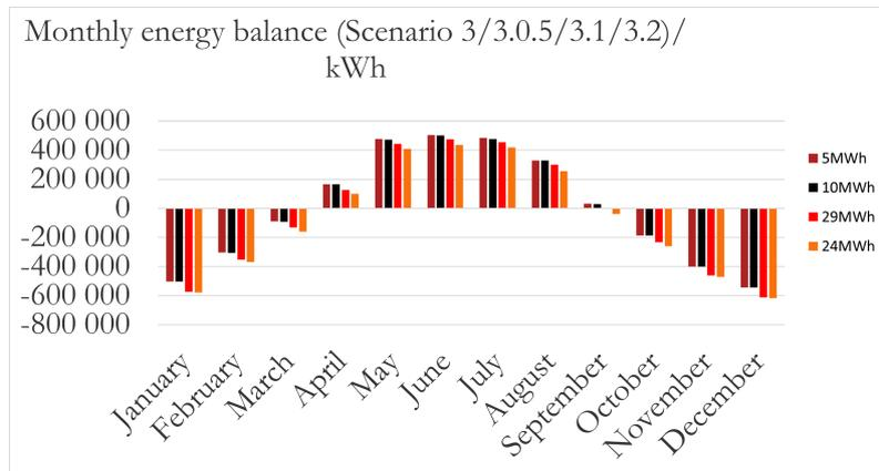
**Figure 4.17:** Monthly energy balance for Scenario 3/3.0.5/3.1/3.2: Current consumption with 5.7 MW PV with 5 MWh, 10 MWh, 29 MWh and 24 MWh battery.
