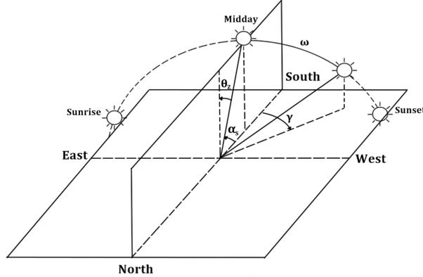
**Figure 3.5:** Definition of hour angle, solar altitude and solar azimuth angle
