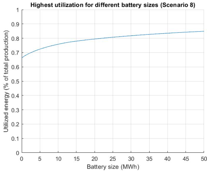
**Figure 4.41:** Highest utilization for each battery size.
