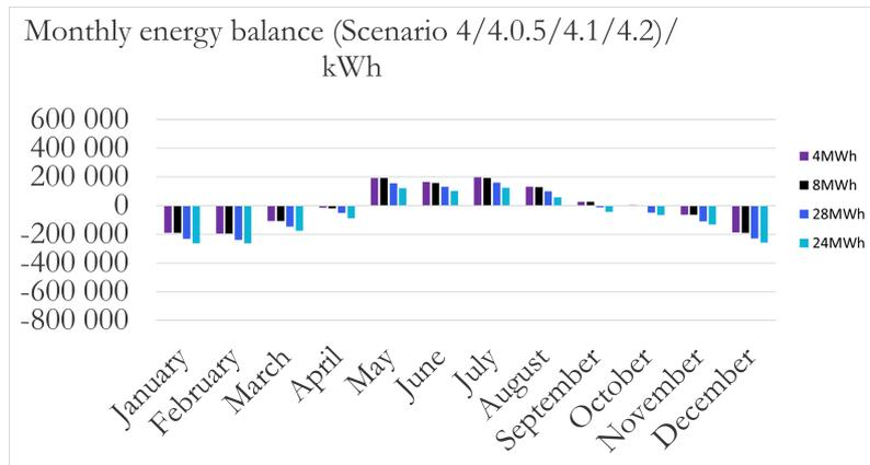
**Figure 4.23:** Monthly energy balance for Scenario 4/4.0.5/4.1/4.2: Current consumption with 2.1 MW PV and 1.0MW Wind with 4 MWh, 8 MWh, 28 MWh and 24 MWh battery.
