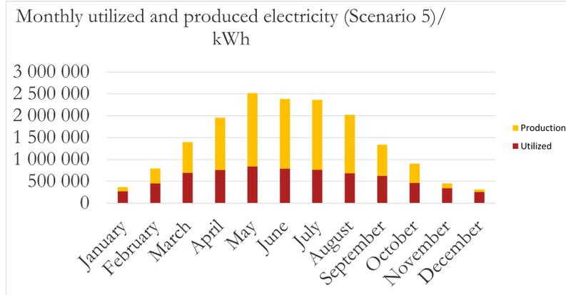
**Figure 4.29:** Monthly production with the amount of utilized electricity of the production for Scenario 5: Shore power with 16.3 MW PV.
