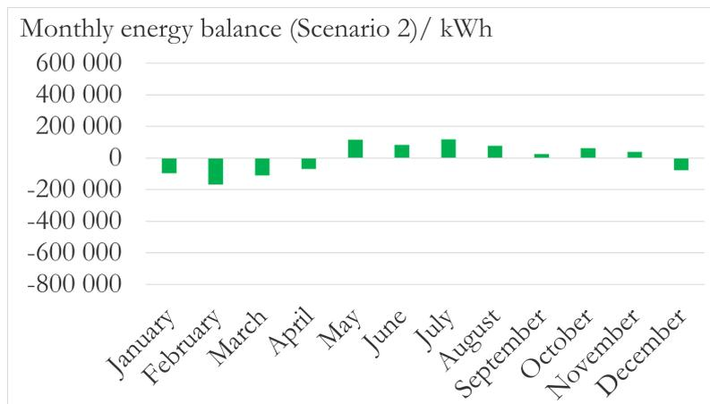
**Figure 4.12:** Monthly energy balance for Scenario 2: Current consumption with 1.1 MW PV and 1.3 MW Wind.
