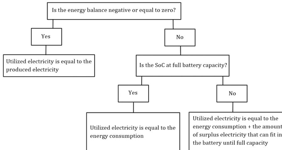
**Figure 3.12:** Sketch of the logic used for utilized electricity in Excel.
