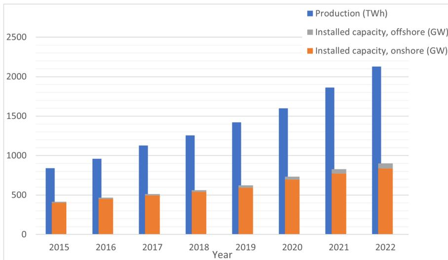
**Figure 2.13:** Global installed capacity and annual production from wind power. Image taken from [29].
