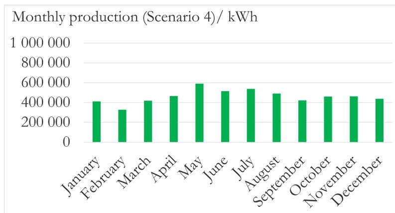
**Figure 4.21:** Monthly production for Scenario 4/4.0.5/4.1/4.2: Current consumption with 2.1 MW PV and 1.0MW Wind with a battery.
