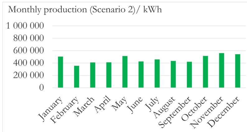
**Figure 4.10:** Monthly production for Scenario 2: Current consumption with 1.1 MW PV and 1.3 MW Wind.
