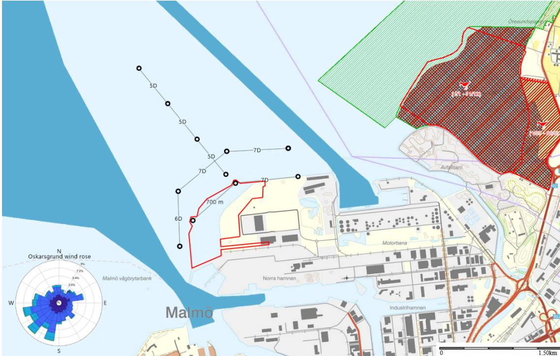
**Figure 4.1:** Some possible siting layouts for 3 MW wind turbines. Hatch marks nature protection areas. Red outline marks the proposed expansion of the harbor. Darker blue is sea lanes. Distances given in meters or rotor diameters,  $D=112$  m. The wind rose for Oskarsgrund is presented as well. Map taken from [39].
