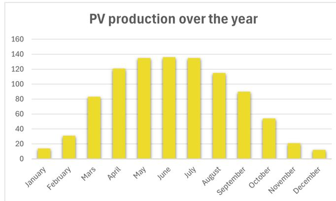
**Figure 2.8:** PV production over the year from a 1kWp system at 35 degrees tilt in Stockholm. Data taken from [14]
