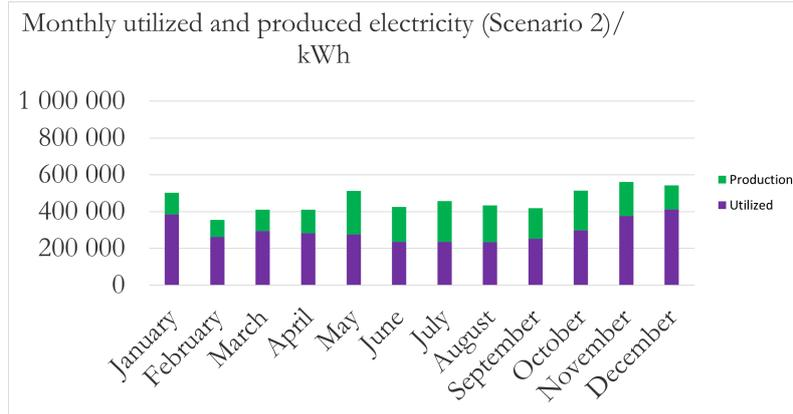
**Figure 4.13:** Monthly production with the amount of utilized electricity of the production for Scenario 2: Current consumption with 1.1 MW PV and 1.3 MW Wind.
