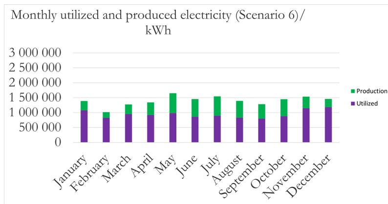
**Figure 4.34:** Monthly production with the amount of utilized electricity of the production for Scenario 6: Shore power with 4.6 MW PV and 3 MW Wind.
