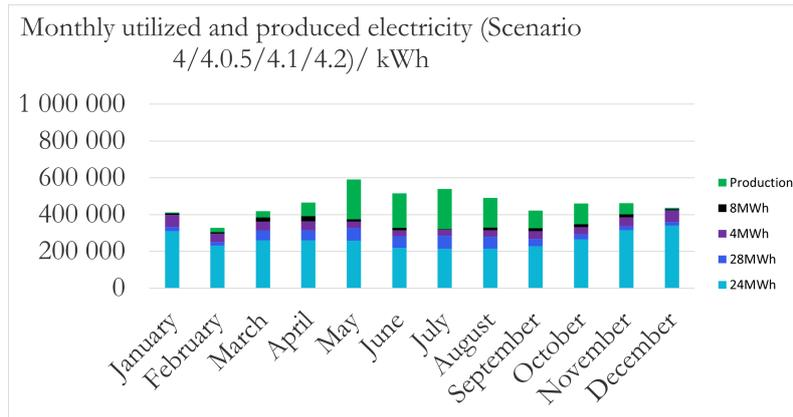
**Figure 4.24:** Monthly production with the amount of utilized electricity of the production for Scenario 4/4.0.5/4.1/4.2: Current consumption with 2.1 MW PV and 1.0 MW Wind with 4 MWh, 8 MWh, 28 MWh and 24 MWh battery.
