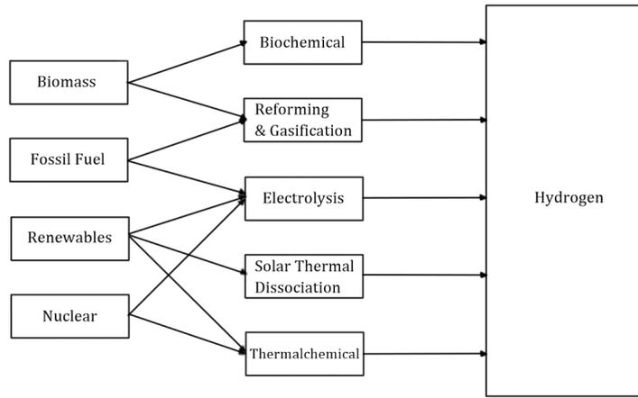
**Figure 2.26:** Production routes of hydrogen.
