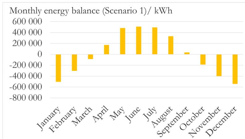
**Figure 4.7:** Monthly energy balance for Scenario 1: Current consumption with 5.7 MW PV.
