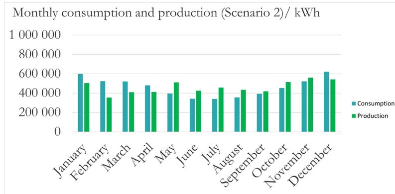
**Figure 4.11:** Monthly production and consumption for Scenario 2: Current consumption with 1.1 MW PV and 1.3 MW Wind.
