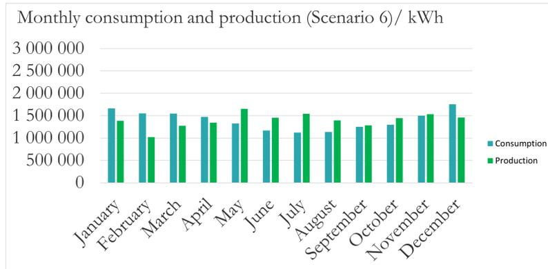
**Figure 4.32:** Monthly production and consumption for Scenario 6: Shore power with 4.6 MW PV and 3 MW Wind.
