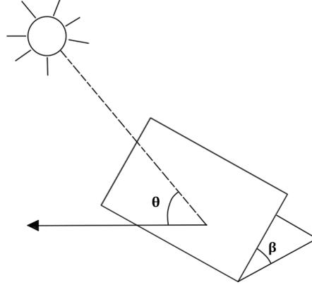
**Figure 3.6:** Definition angle of incidence
